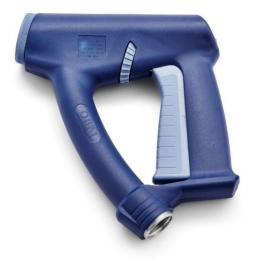
The NiTO II spray gun is thermally insulated and has an adjustable spray angle, from narrow to wide (60°). Suitable for "heavy-duty" applications with a water temperature up to 90 °C and a flow rate of 40 L/min. It is equipped with 3/4" BSP female thread, and the operating handle is lockable to prevent unintended use.
