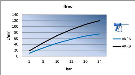
Water flow in I/min when operating lever is fully retracted, depending on pressure
