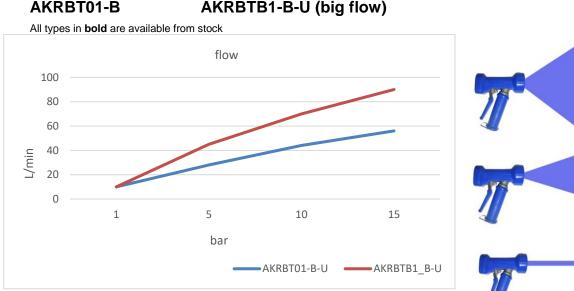
Water flow in I/min when operating lever is fully retracted, depending on pressure
