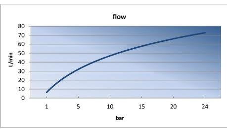
Water flow in I/min when operating lever is fully squeezed, depending on pressure
