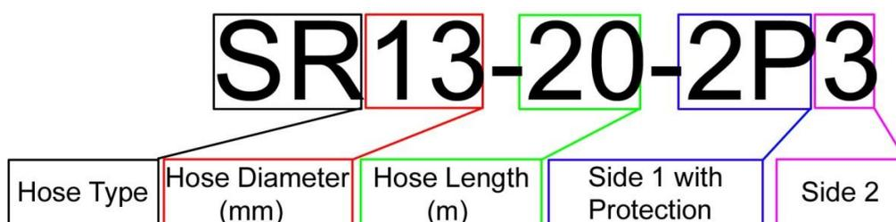
The corresponding numbers for the different hose connections we can mount can be found on the next page.
