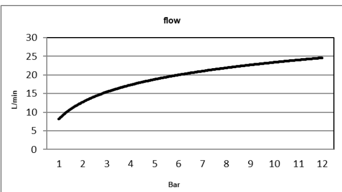
Water flow when trigger is fully squeezed, depending on pressure.
